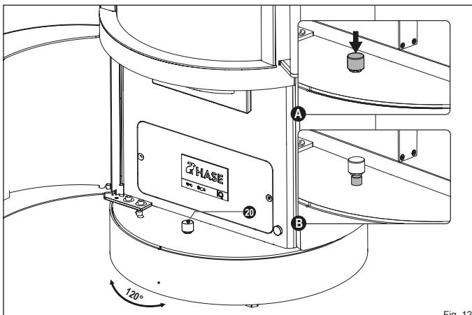
To return the stove to the original position, turn the stove until the notches are flush (Fig. 13):
